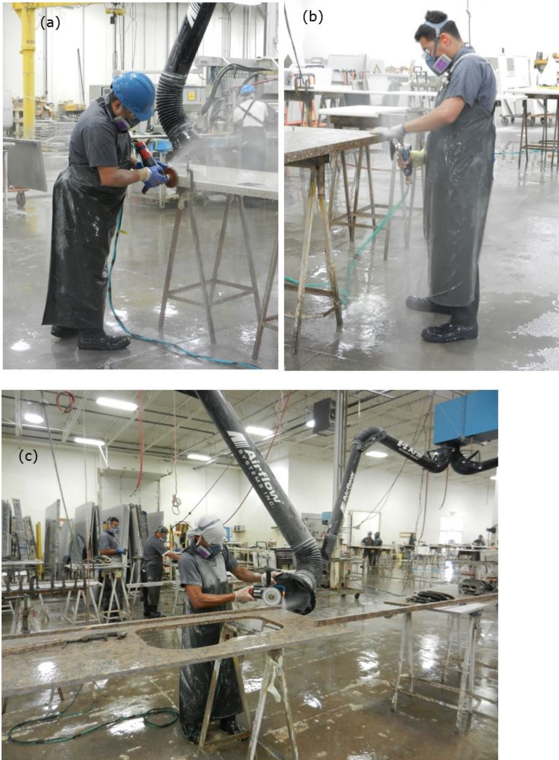
Figure 1 – (a) A worker using a handheld electric wet grinder with a diamond grinding cup wheel in the grinding process; (b) A worker using a handheld pneumatic wet polisher in the
