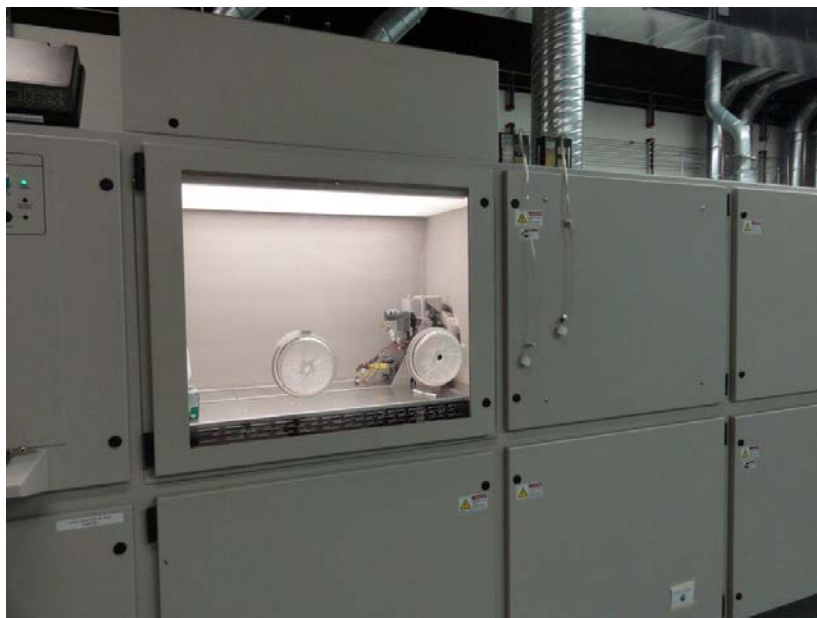
Figure 3. Photograph of the front of the Easy Tube 3000 reactor. The enclosure containing the iris valves is the loading compartment.
