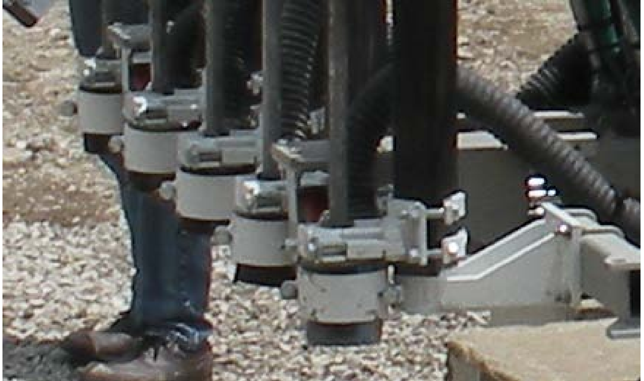
Figure 7 - A Hood Surrounds Each Steel and Bit
