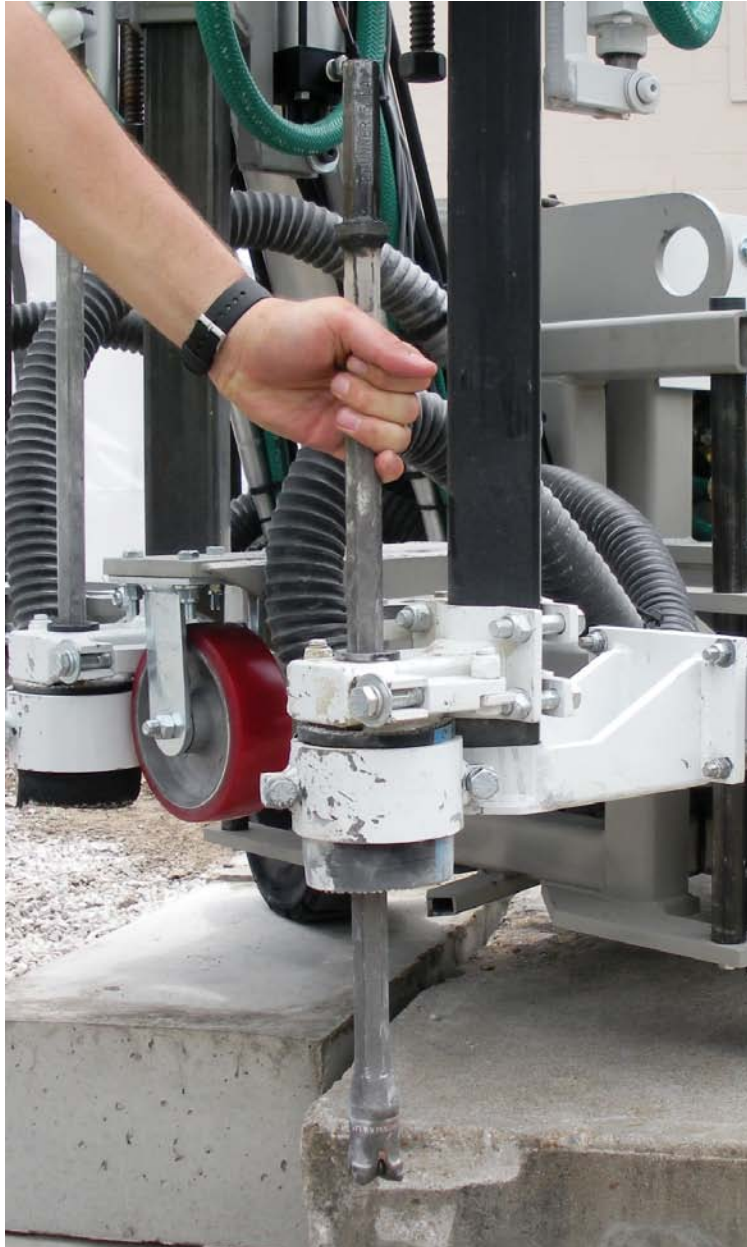
Figure 1 - "H" Thread Steels and 1 \frac{5}{8} -in Diameter Bits Were Used in this Study
