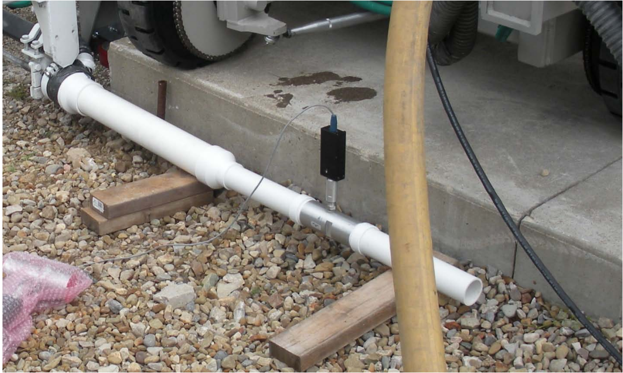
Figure 4 - Set Up for Measuring Bailing Air Flow and Exhaust Air Flow at the Hood
