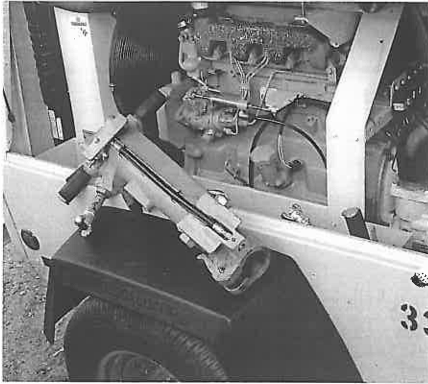
Figure 1: Jackhammer with dust control device.
