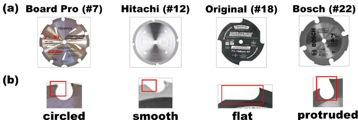
Figure 5. Pictures of (a) saw blades (#7, #12, #18, and #22 from the left) and (b) Enlarged tooth pictures for comparison
