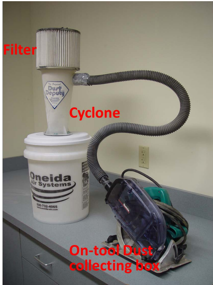
Figure 2. A circular saw (Makita 5057KB) with an on-tool dust-collecting box, and a passive dust collector (a cyclone and a filter cartridge)
