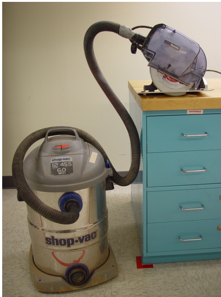
Figure 3. The dust-collecting circular saw and its connection to the shop vacuum.
