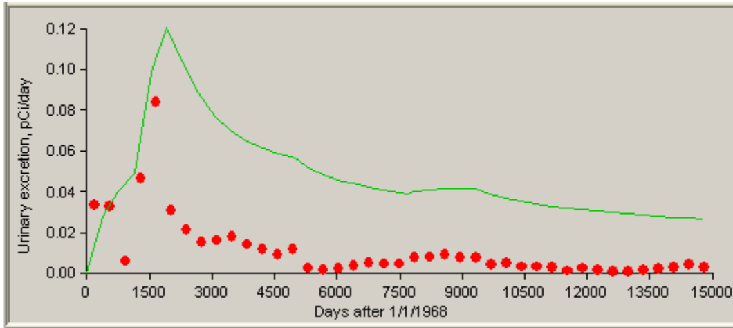
Figure B-17. Predicted 238 Pu bioassay results calculated using IMBA-derived 238 Pu intake rates (line) compared with bioassay results (dots) from all intakes, 84th percentile, type M.
