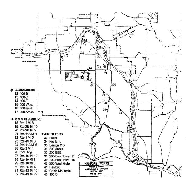
**Figure 4-1.** Locations for environmental monitoring of airborne radioactivity on the Hanford Works in May 1948. Legibility of the source map (<u>HW-9871</u>) was poor, so the legend and location symbols and numbers were redrawn. Also, river monitoring stations were removed from the original figure.
