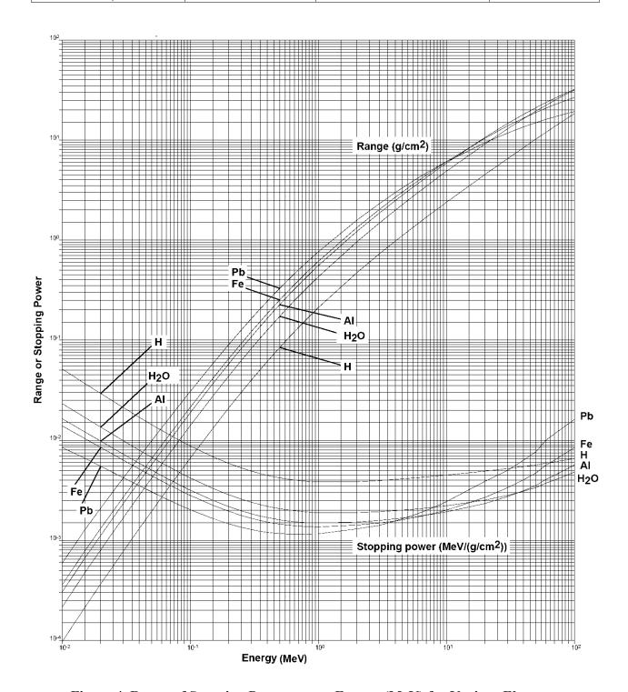
Figure 4. Range of Stopping Power versus Energy (MeV) for Various Elements
