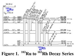
The maximum energy of the  $\beta$  particles is 763.3 | 536.8 = 226.5 keV. About 98% of the  $\beta$ particles have energies below 300 keV. The decay of the excited state of <sup>103</sup>Rh is accompanied by γ emission, with a primary energy of 497 keV.
