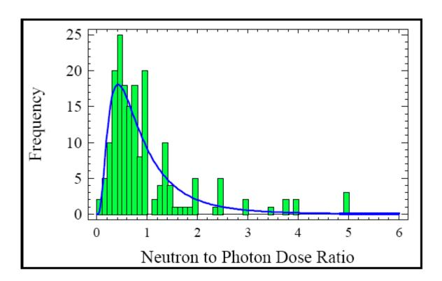
Figure 1. Neutron/Photon Dose Ratio Distribution of Hanford Plutonium Facility Workers
