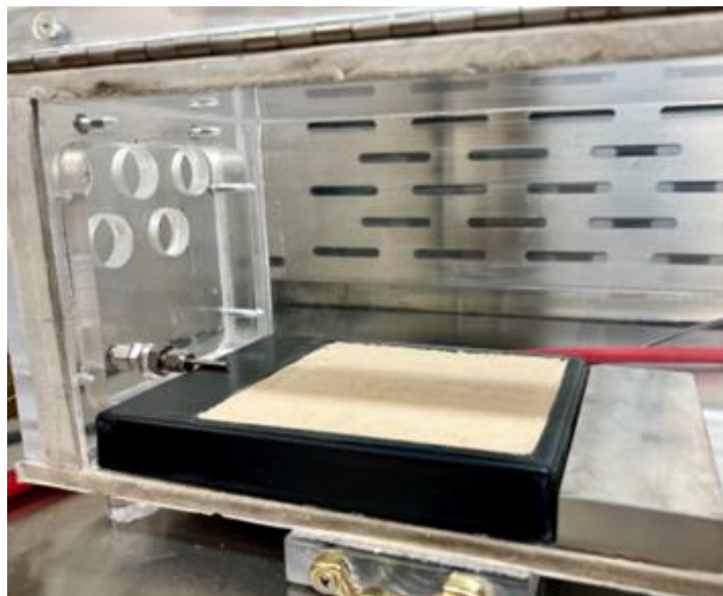
Figure 8. Dispersion nozzle, test sample tray (pre-loaded with mineral dust), and ballast weight to prevent the tray shifting during an experiment (photo provided by D.E. Evans, NIOSH). A series of five holes in the chamber, situated above the nozzle, introduce laboratory air for dust transport. The front hinged lid of the chamber is opened for clarity. The dust sample tray is 190 mm long.
