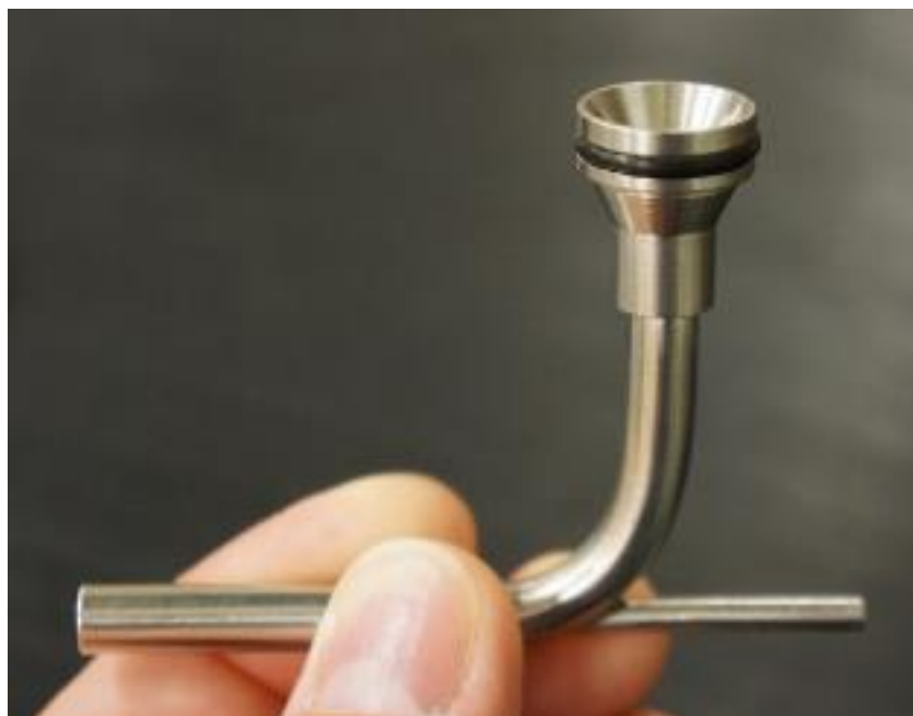
Figure 5. The UNC Venturi dispersion nozzle with lid removed (photo provided by D.E. Evans, NIOSH). The nozzle is fabricated from stainless steel. The O-ring seal for the lid (removed) is visible at the funnel. The length of the nozzle (from left to right) is 72 mm. The left portion of the nozzle is inserted into the glass containment chamber through a rubber grommet.
