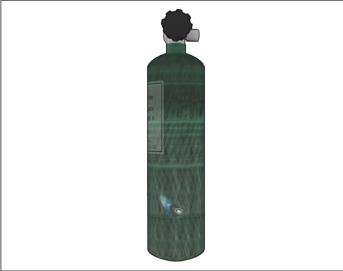
Figure 27. A dent on the oxygen cylinder shown on the back side.
