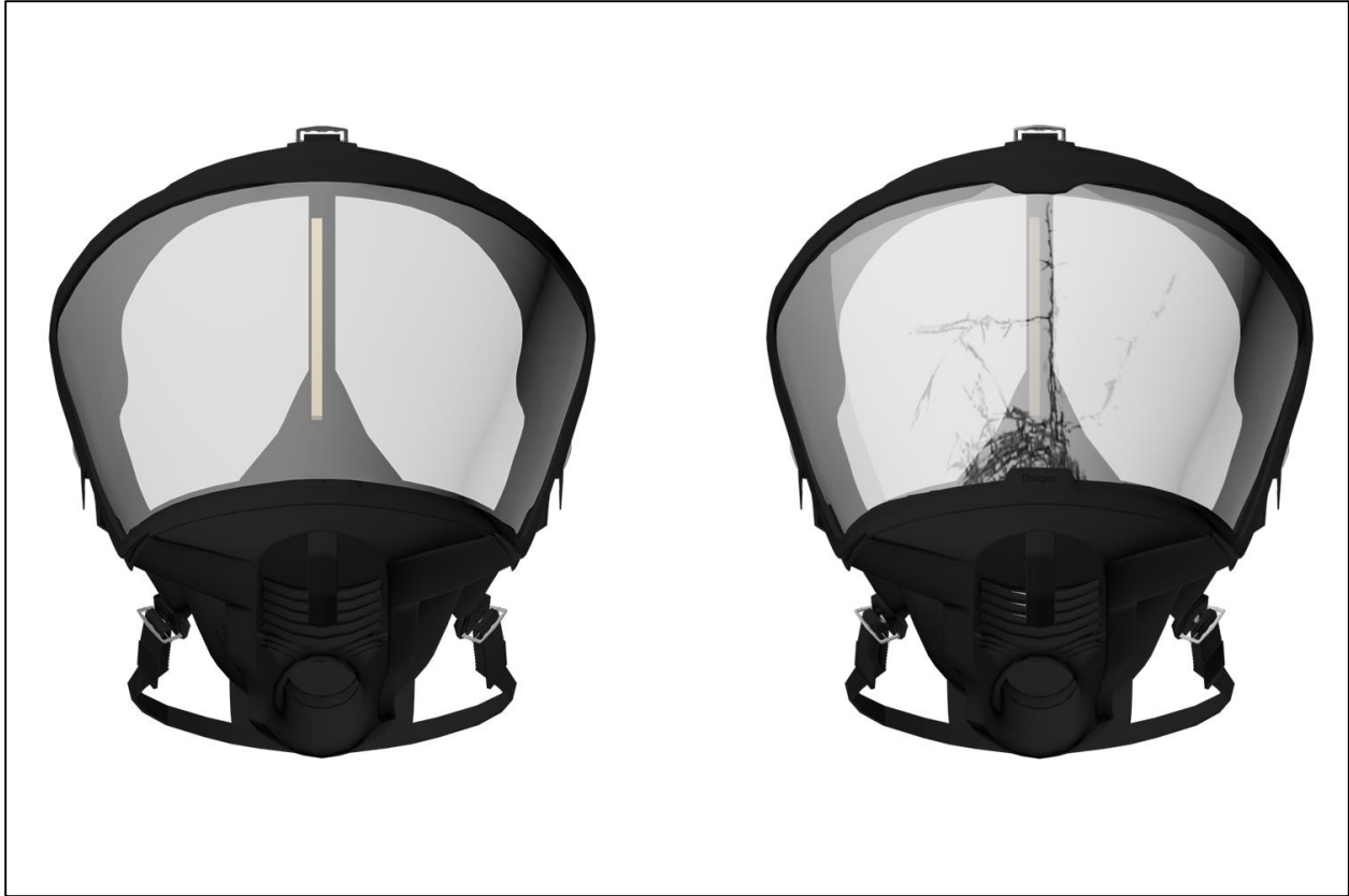
Figure 22. Cracked glass on the full face mask is shown on the right. The nonflawed full face mask is shown on the left.
