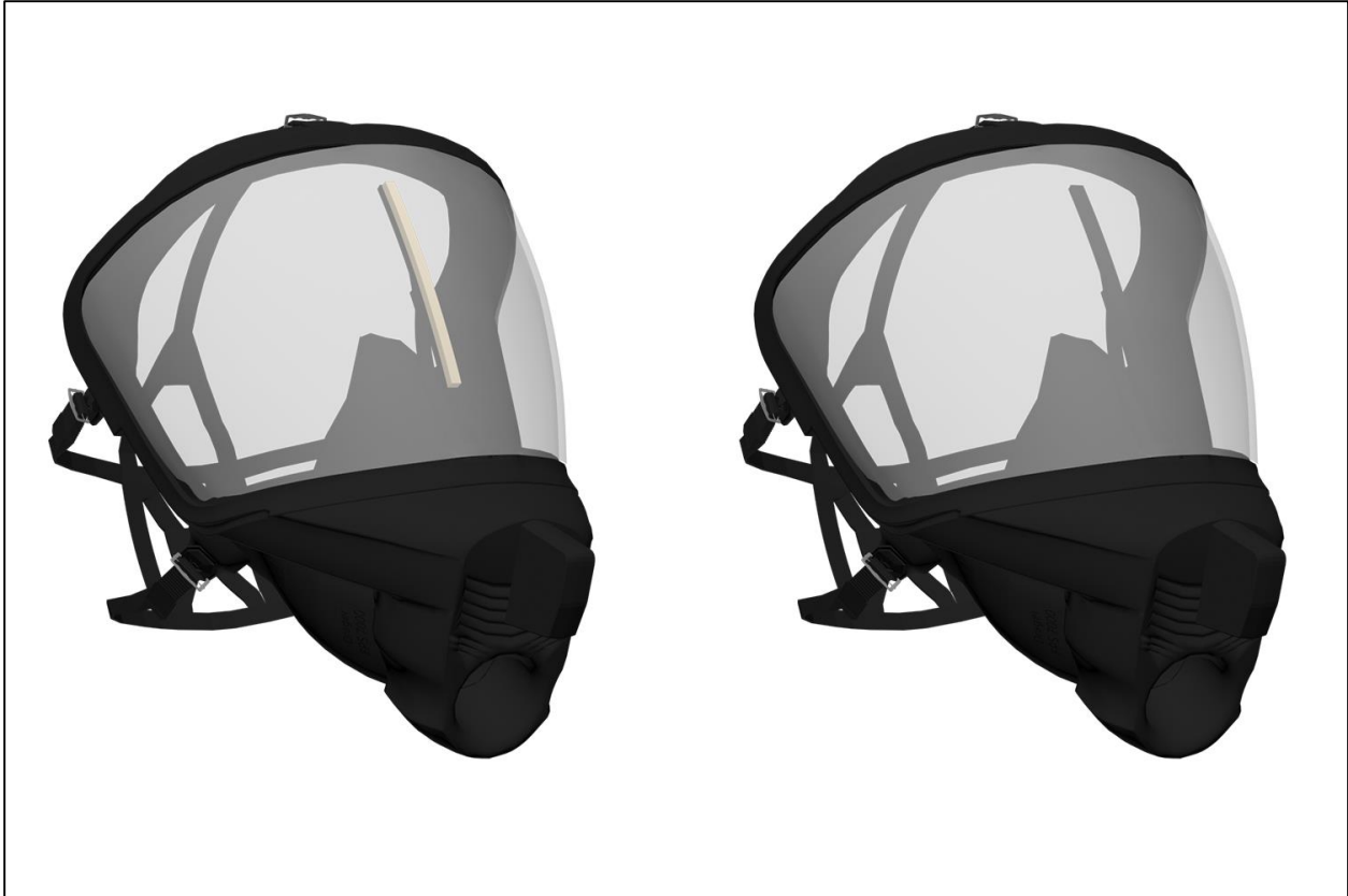
Figure 23. A missing wiper on the full face mask shown on the right. The nonflawed full face mask is shown on the left.
