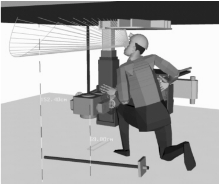
Figure 2. Vision cone in the roof bolter model
