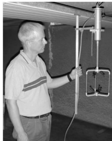
Figure 3. Three-axis ultrasonic anemometer.
