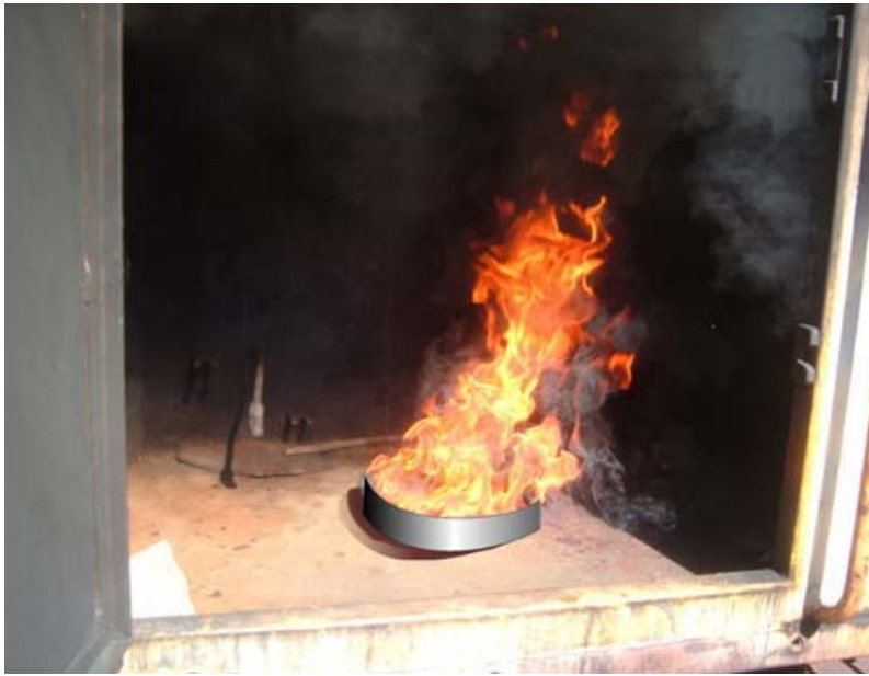
Figure 4. Prelit fuel tray fires (32 kW: 250 ml diesel and 250 ml gasoline contained in a 23 cm dia fuel tray).
