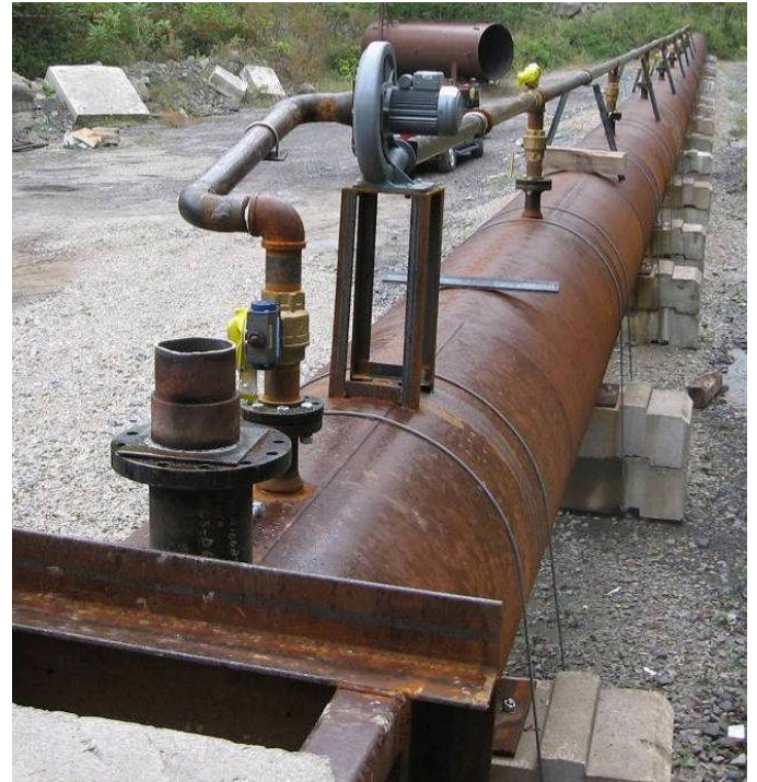
Figure 8. 1,048-mm-diameter (42 in) gas explosion tube at NIOSH Lake Lynn Laboratory.
