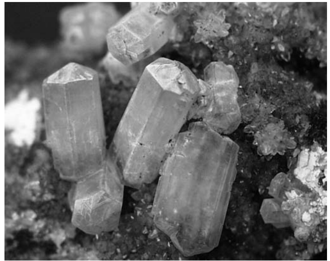
Figure 15 — Ettringite mineral. Ettringite is a key component that provides high yield (more water than solids) and facilitates fast setting and high strength.
