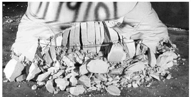
Figure 21 —The final product produced from CSA grout is light in color and lightweight.
