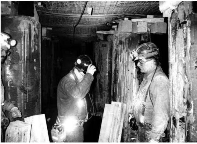
Figure 1 — The Can is a commonly used tailgate support in the United States.
