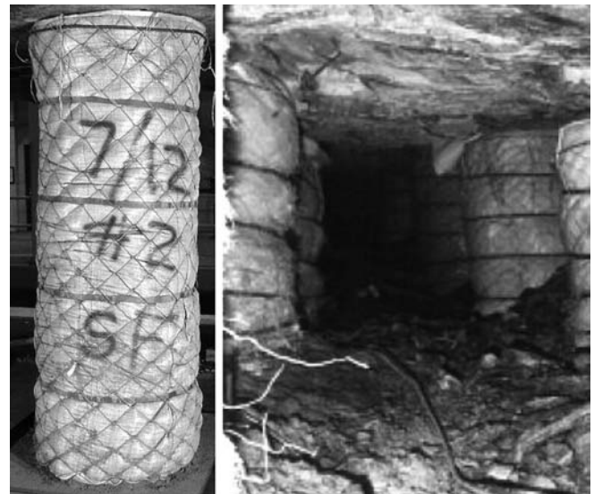
Figure 9 — Mesh Pack pumpable support showing laboratory test specimen on left and in mine trials on right (courtesy of Strata Products USA).
