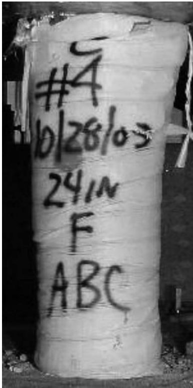
Figure 14 — Photo of Tekpak P pumpable support after 150 mm (6 in.) of convergence carrying a load of about 45 t (50 st).
