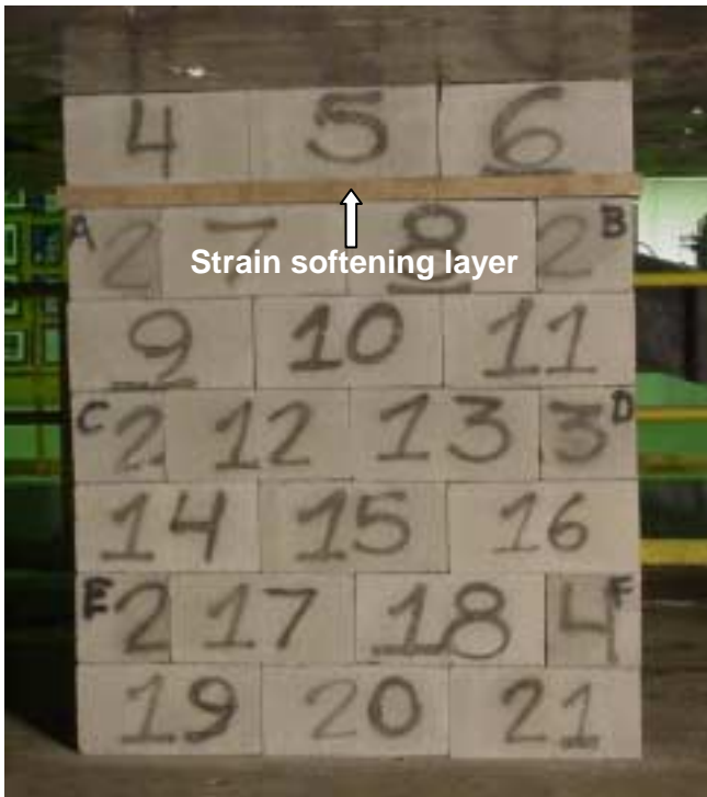
Figure 6. Seven-course concrete block wall dry-stacked with one layer of wood below the top row of blocks and tested in the MRS.
