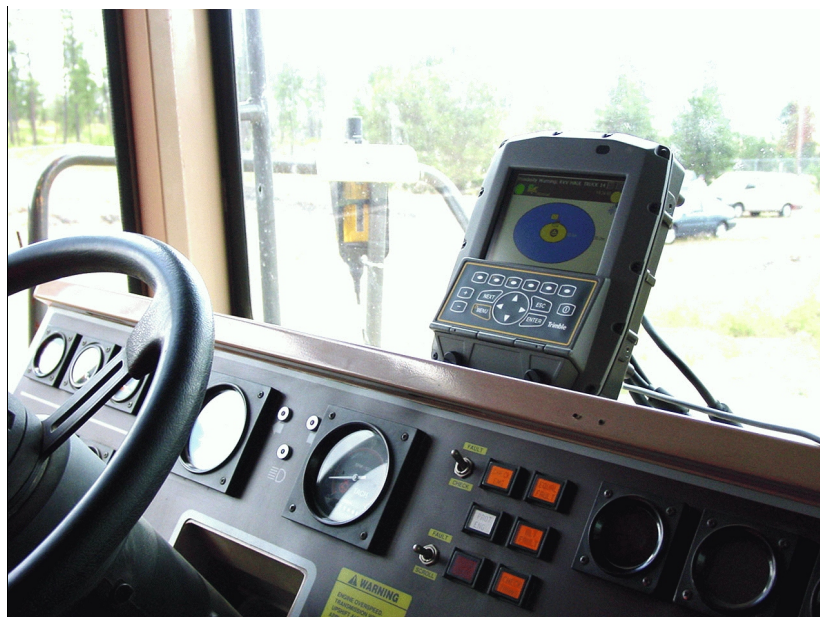
Figure 7. Graphics display for GPS-based collision warning system.
