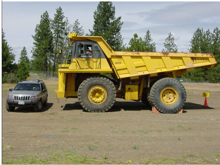
Figure 6. Tests of collision warning system using GPS and peer-to-peer communication between dump truck and passenger vehicle.
