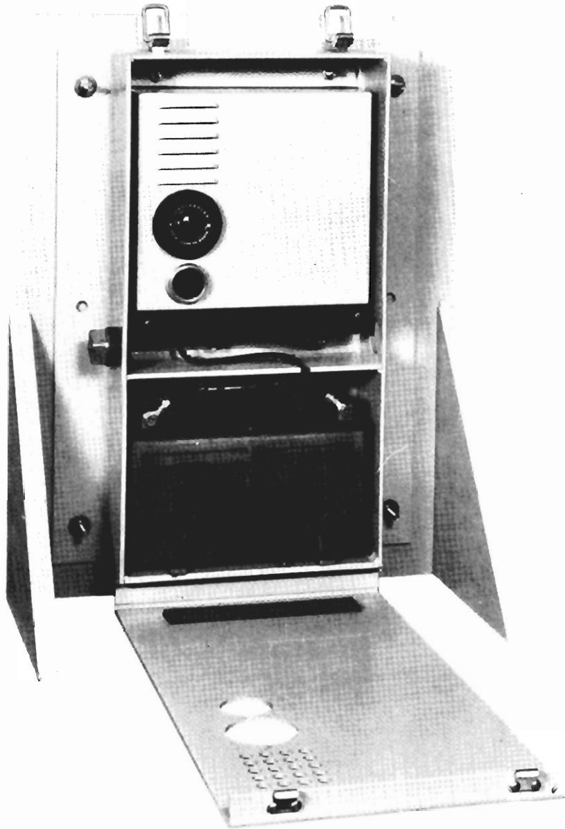
Figure 5-37. Cage Transceiver and Battery in Protective Enclosure.
