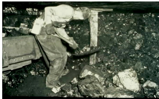
Figure 4. Hand loading with a safety post.
