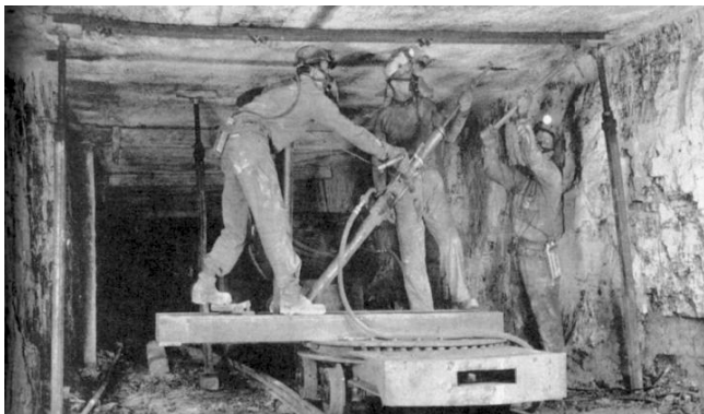
Figure 17. Dry drilling using respirators for dust protection.
