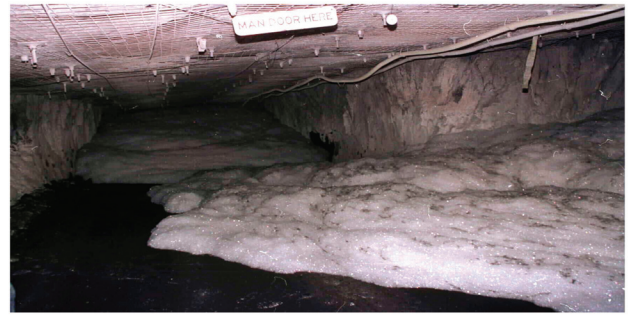
Figure 9 — Leading edges of foam plug in entry No. 2 and from crosscut on right.
