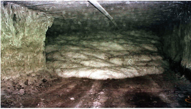
Figure 6 — Leading edge of foam plug in No. 3 entry, first crosscut on left.
