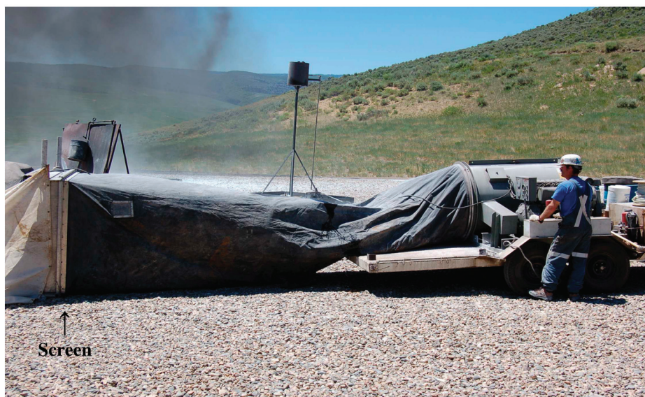
Figure 1 — Jamison 510 m 3 /min (18,000 cfm) high-expansion foam generator with attached expandable shroud and screen.
