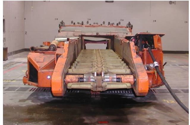
Figure 2: 14CM-9 Continuous Mining Machine in Reverberation Chamber
