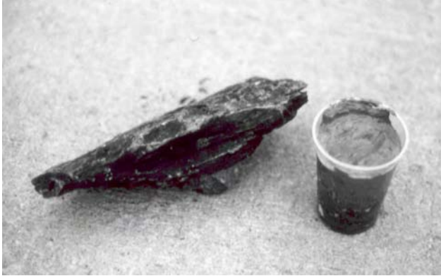
Figure 1.—Effect of water on a moisture-sensitive shale.
