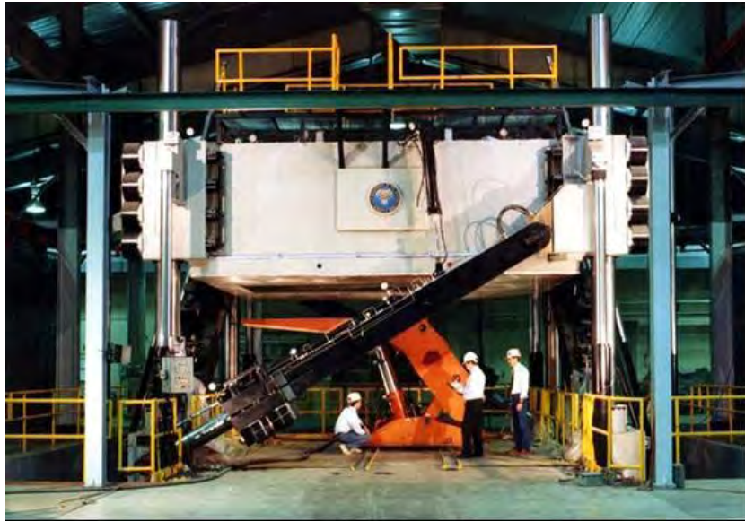
Figure 3 – NIOSH's Mine Roof Simulator (MRS) [17].
