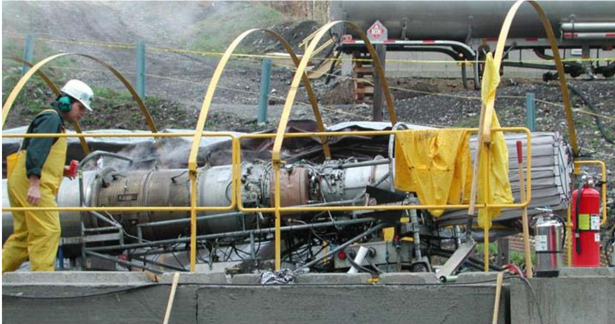
Figure 3. GAG 3A jet engine and afterburner, Loveridge Mine.
