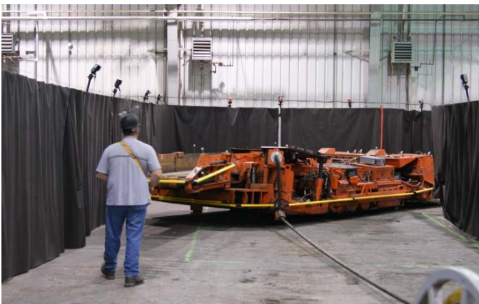
Figure 6. Tramming test of iPD in simulated mine.
