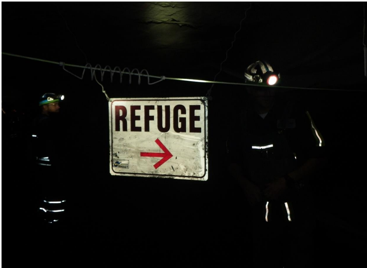
Figure 19. Reflective signage indicating the location of an RA in an underground coal mine.
