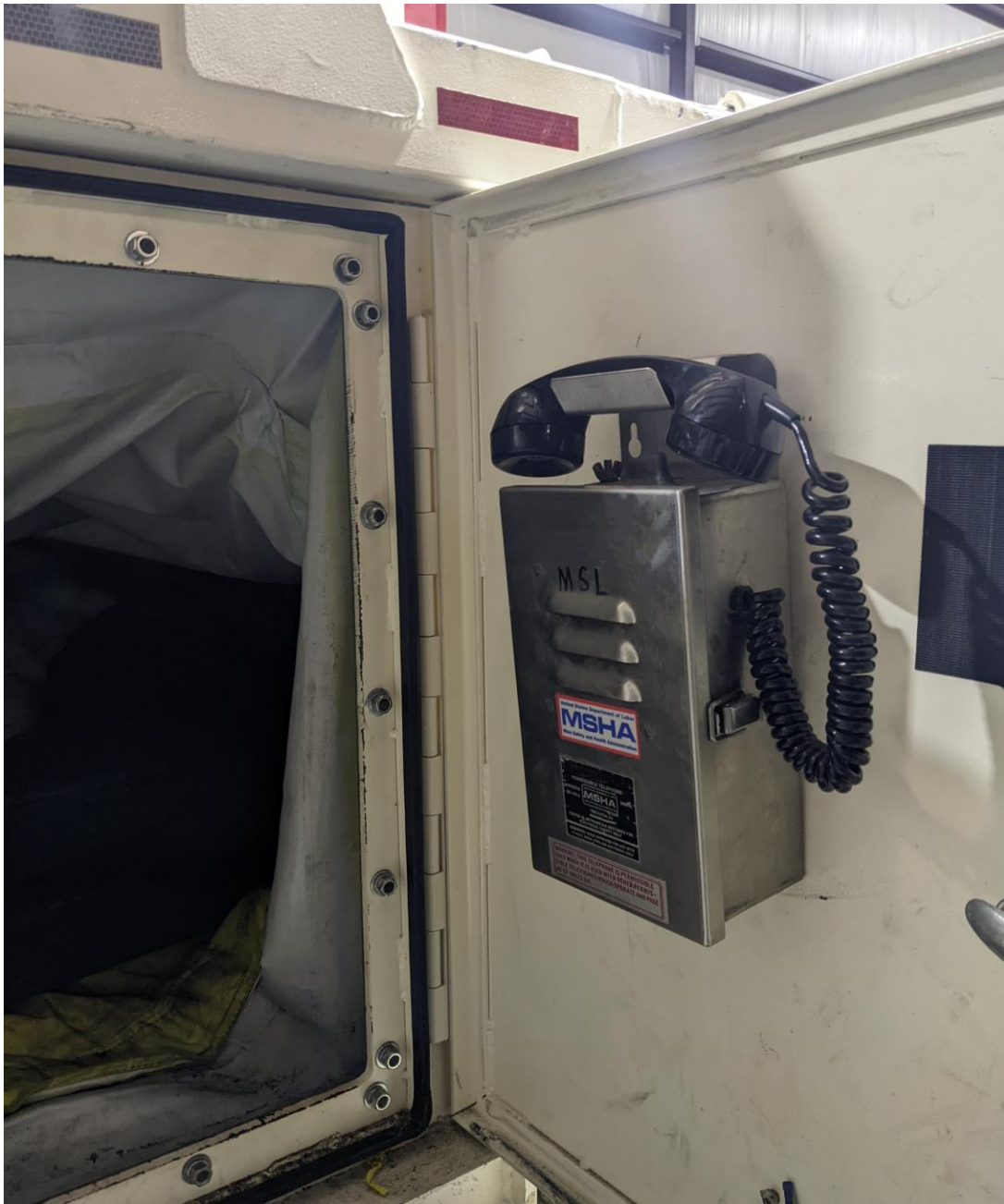
Figure 18. A mine phone affixed to the inside of a refuge alternative door.
