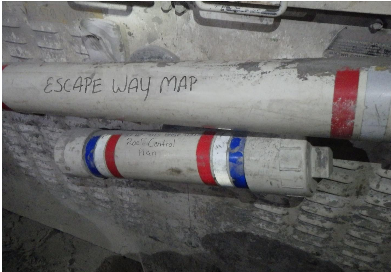
Figure 5. Escapeway map and roof control plan stored in PVC pipes at a mine's designated meeting place.
