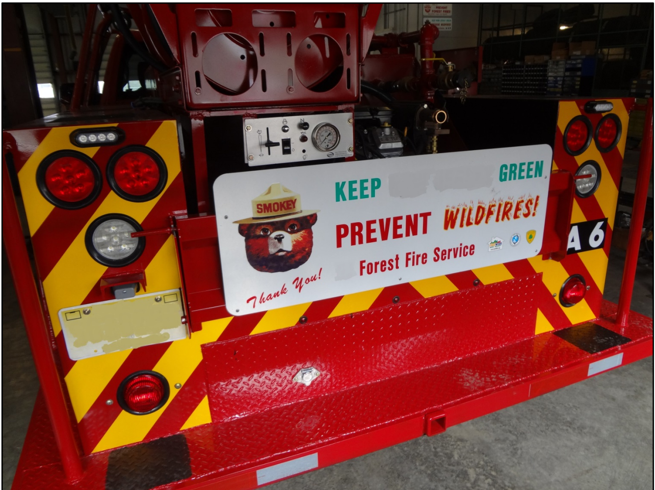
Photo 4. Another view of the new engine. Note the high-visibility chevrons added on the rear of the engine for increased conspicuity.
