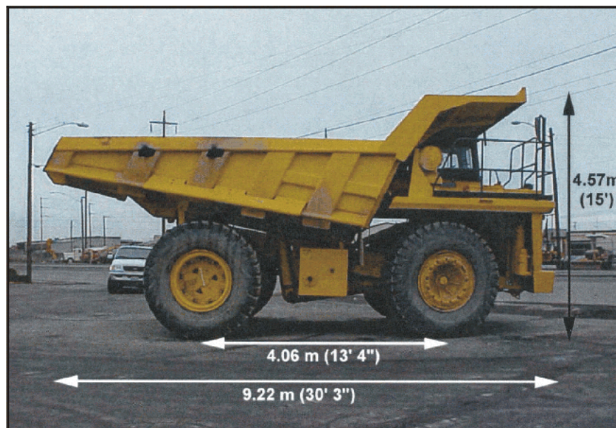
Figure 4.—Komatsu 210M 50-ton-capacity dump truck used as test platform.
