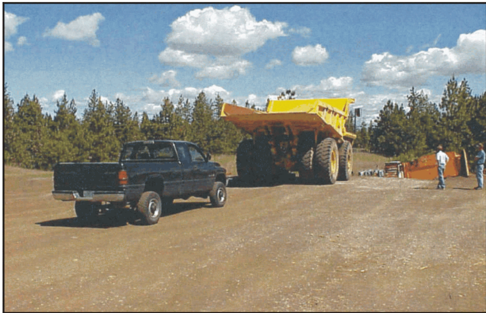
Figure 6.—Test configuration using pickup as obstacle.
