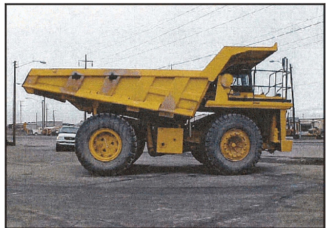
Figure A-2.—Fifty-ton-capacity Komatsu dump truck.
