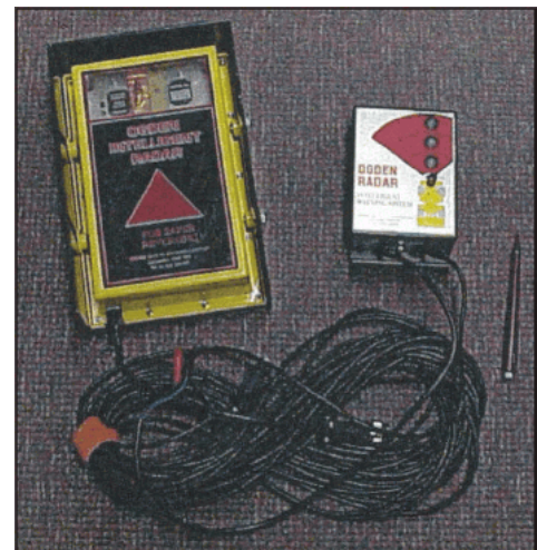
Figure 2.—FMCW radar-based collision warning system manufactured by Ogden Safety Systems showing antenna and electronic enclosure (left) and alarm display (right).
