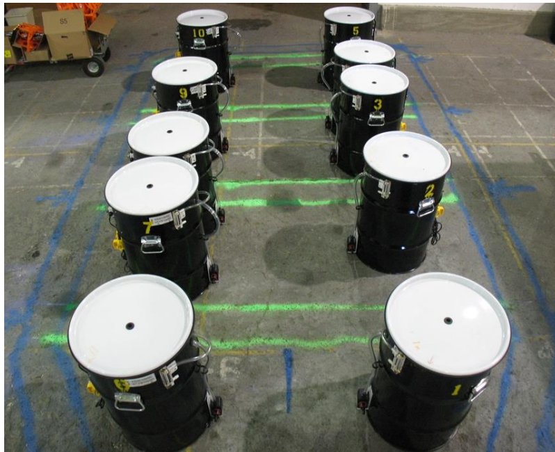
Figure 6. Layout of simulated miners within outline representation of the tested RA (lines represent support tubes).
