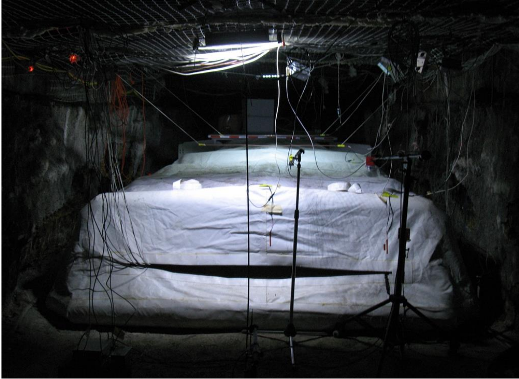
Figure 11. RA set up for apparent temperature testing in the SRCM.
