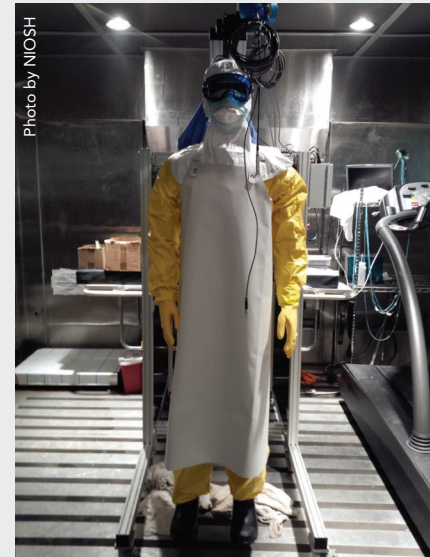
NIOSH sweating thermal manikin with the PPE ensemble commonly used by Médecins Sans Frontières (Doctors without Borders) for high exposure areas. This PPE ensemble includes a TyChem C coverall (a type of limited-use Chemical Protective Coverall), a custom-made Tyvek hood with integrated surgical mask, rubber apron, respirator, goggles, rubber gloves, and rubber boots. Photo by NIOSH.
