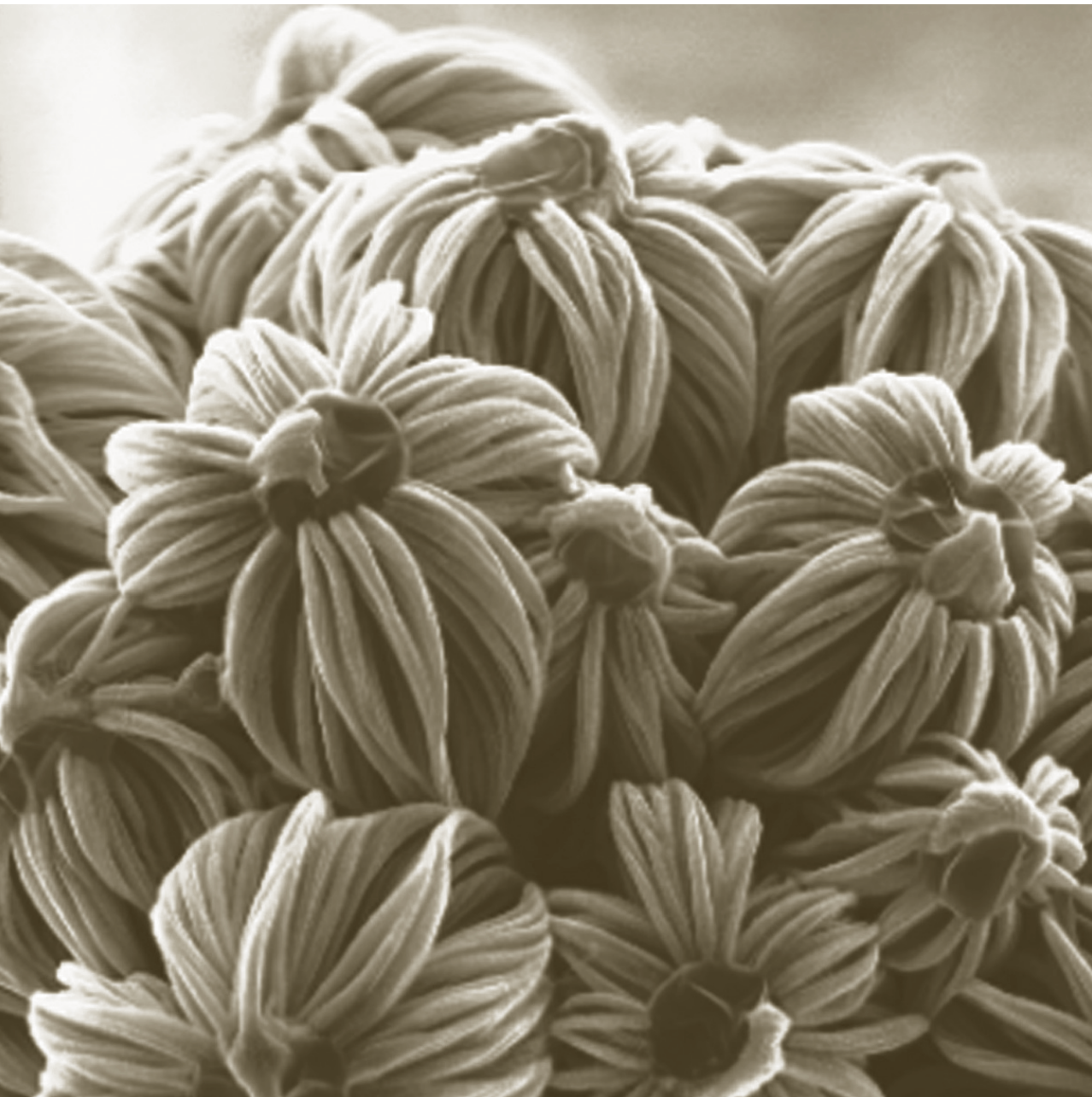
Flower Bouquet, a 3-D nanostructure grown by controlled nucleation of silicon carbide nanowires on Gallium catalyst particles. As the growth proceeds, individual nanowires 'knit' together to form 3-D structures. Credit: Ghim Wei Ho and Professor Mark Welland, Nanostructure Center, University of Cambridge. Courtesy: National Science Foundation
