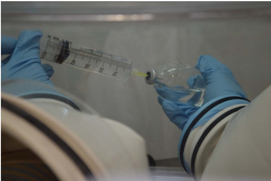
Figure 3. Photograph showing the transfer of 45 mL of hazardous drug surrogate from a septum-capped vial into one of two 60 mL syringes (no CSTD shown). (Photo Credit: NIOSH)
