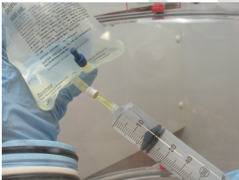
Figure 2. Photograph showing the injection of one of two 45 mL doses of hazardous drug surrogate into a 500 mL 0.9% sodium chloride IV bag (no CSTD shown). (Photo Credit: NIOSH)
