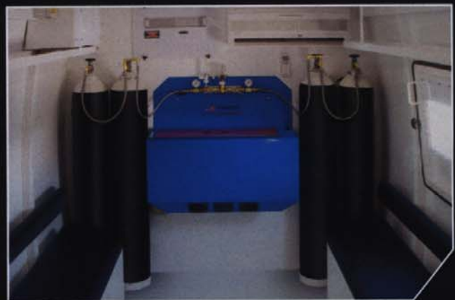
Air Scrubber & Oxygen System
