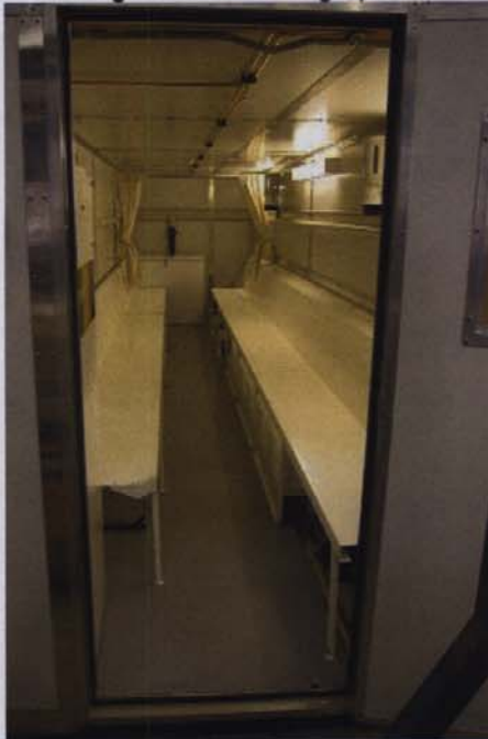
Rescue Chamber designed specifically for underground tunnelling operation
