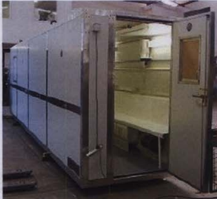
Rescue Chamber designed specifically for underground tunnelling operation
