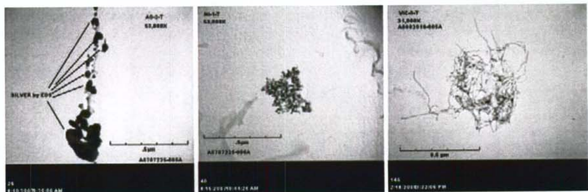
Figure 7–2. Photomicrographs of airborne engineered nanomaterials (airborne samples of engineered nanoparticles of silver, nickel, and MWCNT analyzed by TEM and EDS)
