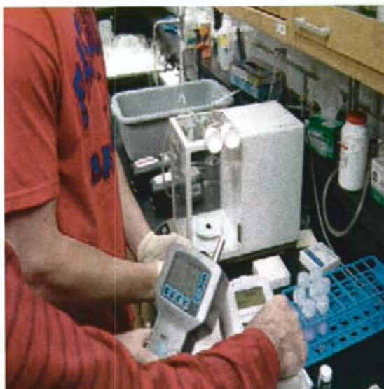
Figure 7-3. Combined use of the OPC, CPC, and two filter samples to determine the presence of nanomaterials
