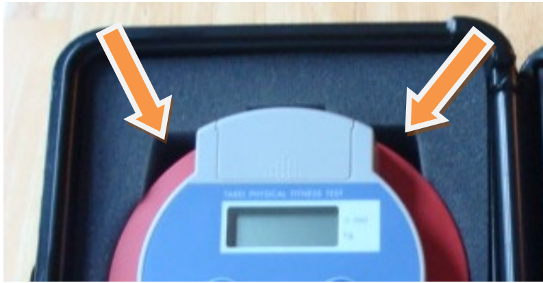
Figure 2-8. Storing dynamometer batteries
