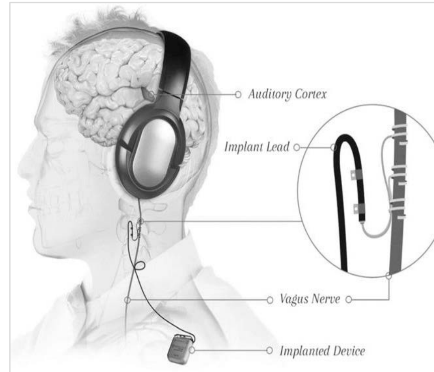
Setup pairing Vagus Nerve Stimulation (VNS) with tones. The inset shows the electrode lead wrapped around the vagus nerve. A pulse generator is implanted under the chest wall. Image courtesy of MicroTransponder, Inc.
