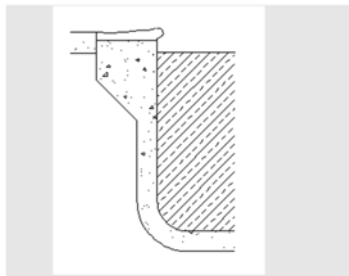
Figure 4.5.12.1: Plumb Pool Walls: Cross-Section
