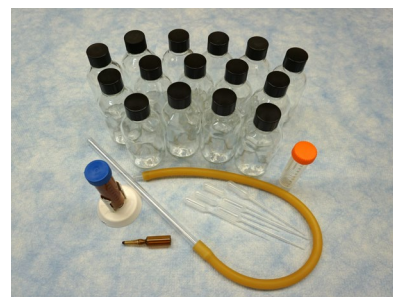
The CDC bottle bioassay kit is used to determine whether a particular insecticide is effective against local mosquito species.
